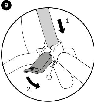
Insert the push rod into the seat retainer and lock into place. Ensure that the locking mechanism (spring) locks in correctly (!).
