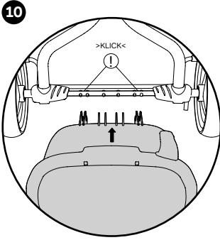
Position the recess on the rear axle until it locks into place.
