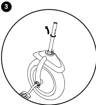
Remove transport lock (cardboard, rubber band) and take off the washer.
