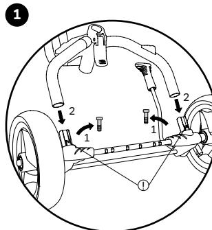
Undo screws and insert rear axles into frame.
