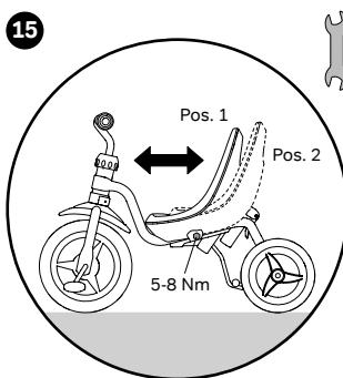
The seat position can be adjusted into myriad positions by loosening the screw somewhat. Afterwards, tighten the screw sufficiently.
