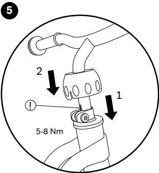
Slide the handlebar all the way onto the fork shaft, and tighten the screw. Firmly press down on the spherical cap until it snaps into position. Align the slot in the handlebar with the rear (!).
