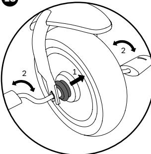
Deactivate the freewheel so that the child can step on it too: to do so, push the locking ring against the rim until it locks. Turn crank slightly, as it makes locking easier.
