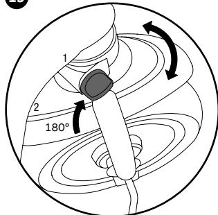
Turn rotary knob 180° so that handlebar locking is activated or deactivated.
