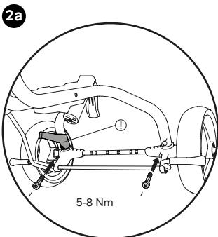
Only on Ceety Comfort model: guide left screw through the parking brake (!) opening and tighten.
