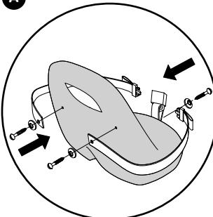
Lock the pierced ends of the belt to the tricycle seat using the screws in the size provided.
