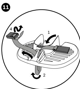
Pull the enclosed belt through the footrest, then through the belt bar.
