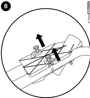
Unscrew screws from the seat retainer.
