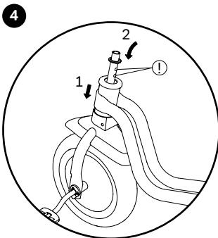
Slide the steering tube onto the fork shaft, until it reaches the stop... Replace the washer again. Align the lug on the handlebar to the rear (!).
