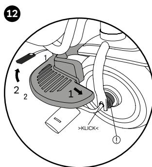
Position the footrest on the crank and attach the belt to the frame. If using the footrest, the freewheel must be enabled - pull the lock ring away from the rim (!).
