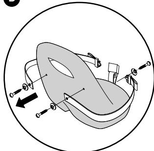
Remove the belt by loosening the screws.
