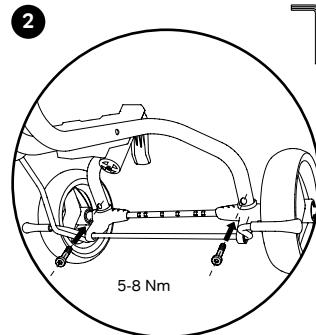
Insert screws and tighten.
